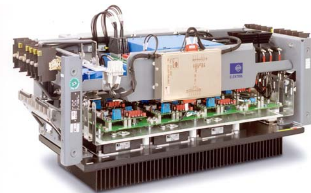
Figure 10. Inverter Bombardier TC 3200 for high-power locomotives.
