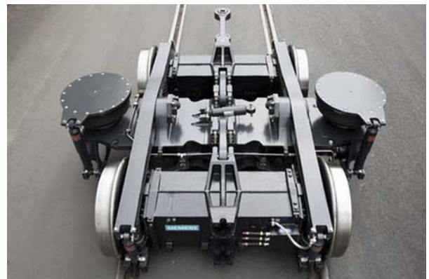
Figure 11. SYNTEGRA bogie with two gearless PMSM.
