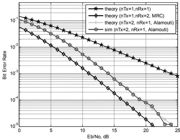
Fig. 3 BER vs Eb/No for BPSK modulation with Alamouti STBC(Rayleigh channel)
