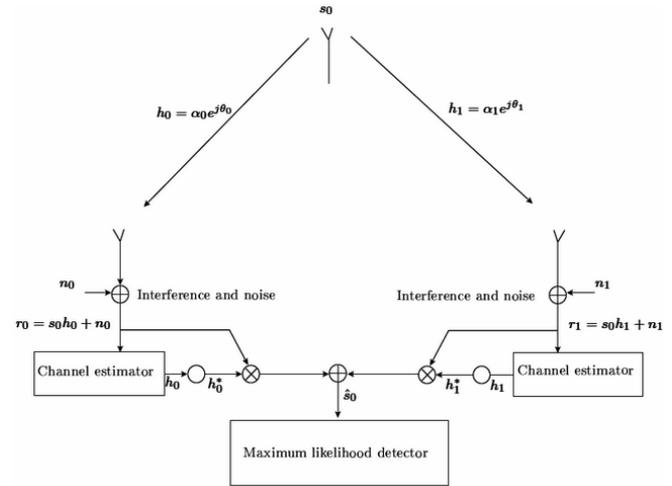
Fig. 1 Maximum ratio receive combining
