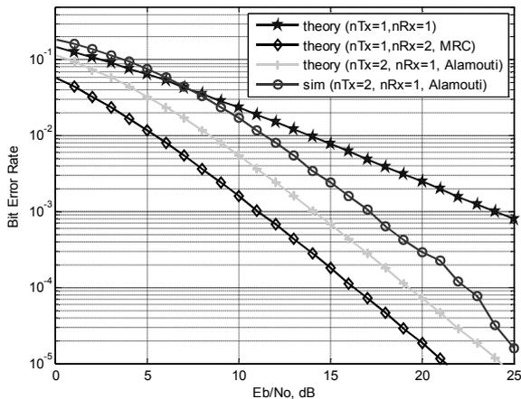
Fig. 4 BER vs Eb/No for QPSK modulation with Alamouti STBC(Rayleigh channel)
