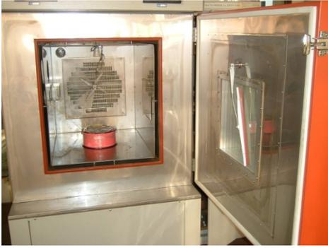
Figure 2 Optical fiber coil in device with artificial atmosphere
