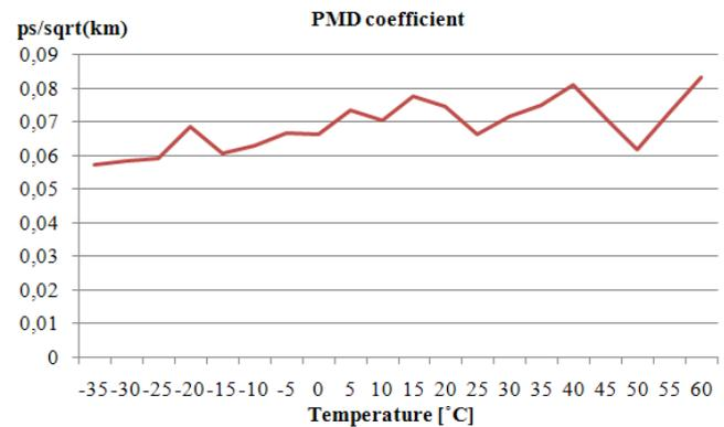
Figure 8 Graph of polarization mode dispersion coefficient change
