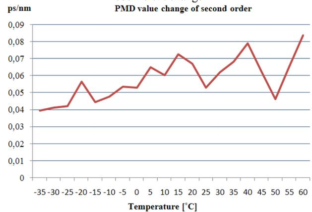
Figure 9 Graph of polarization mode dispersion value change of second order
