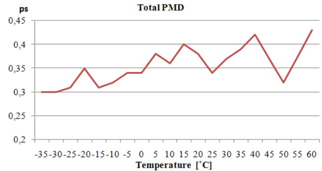
Figure 7 Graph of polarization mode dispersion value change with temperature growth
