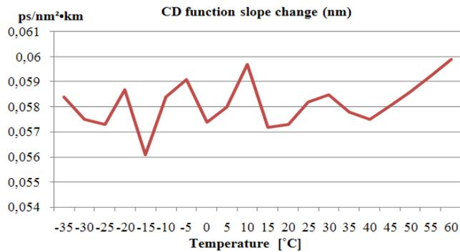
Figure 5 Graph of chromatic dispersion function slope change
