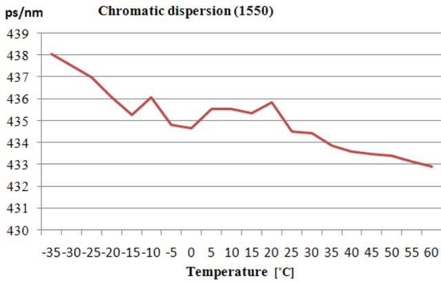
Figure 3 Graph of chromatic dispersion change with temperature growth
