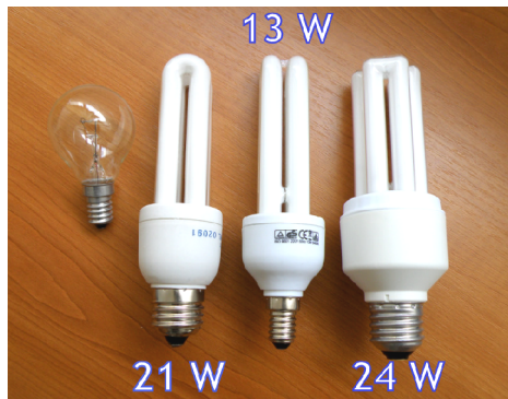
Figure 2 - CFL tested: 13 W, 21 W and 24 W
