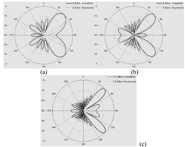
Fig. 5. Radiation pattern of a (a) 6, (b) 8, and (c) 12 elements antenna array with  $\varphi_0$  equal to  $45^\circ$ .
