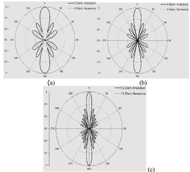
Fig. 4. Radiations pattern of a (a) 6, (b) 8 and (c) 12 elements antenna array with  $\varphi_0$  equal to  $0^\circ$ .
