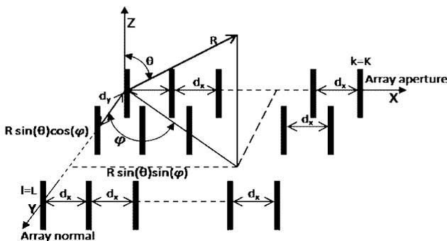
Fig. 2. Schematic representation of the planar antenna array consisting of  $K \times L$  elements and the coordinate axes.
