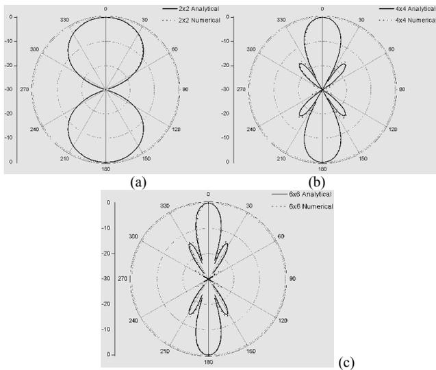
Fig. 7. Radiation pattern of a of a (a) 2x2, (b) 4x4, and (c) 6x6 elements planar antenna array with  $\varphi_0$  equal to  $0^\circ$ .
