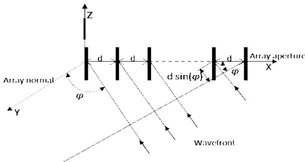
Fig. 1. Schematic representation of the linear antenna array and the coordinate axes.
