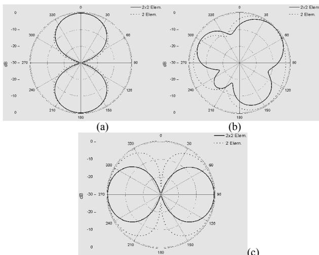
Fig. 10. Radiation pattern of a 2 elements antenna array and a 2x2 elements planar antenna array for (a) 0°, (b) 45°, and (c) 90° degree scanning angle
