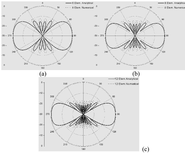
Fig. 6. Analytical and numerical radiation pattern of a (a) 6, (b) 8, and (c) 12 elements antenna array with  $\varphi_0$  equal to  $90^\circ$ .
