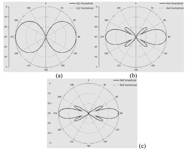
Fig. 9. Radiation pattern of a of a (a) 2x2, (b) 4x4, and (c) 6x6 elements planar antenna array with  $\varphi_0$  equal to  $90^\circ$ .
