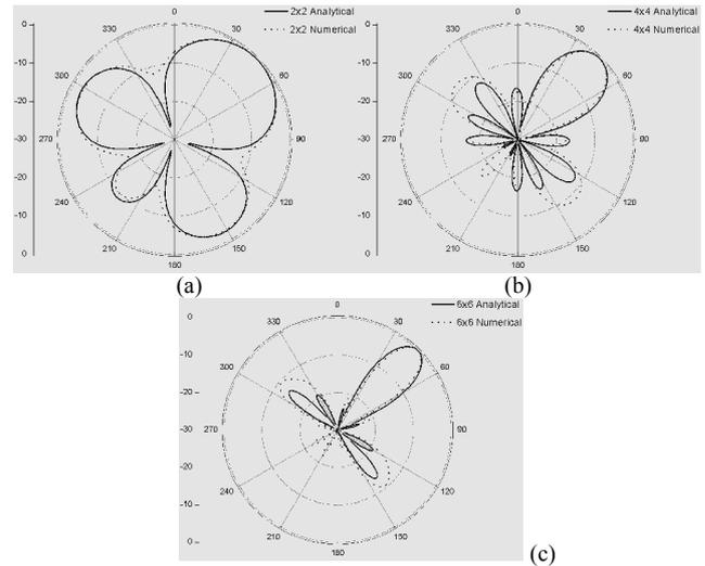
Fig. 8. Radiation pattern of a of a (a) 2x2, (b) 4x4, and (c) 6x6 elements planar antenna array with  $\varphi_0$  equal to  $45^\circ$ .
