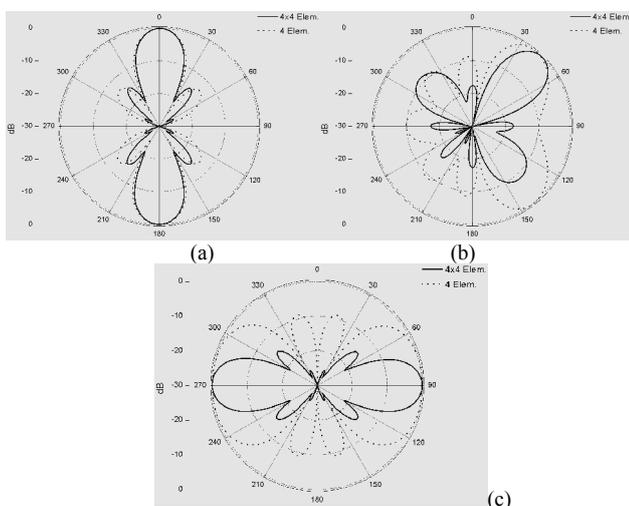
Fig. 11. Radiation pattern of a 4 elements antenna array and a 4x4 elements planar antenna array for (a) 0°, (b) 45°, and (c) 90° degree scanning angle
