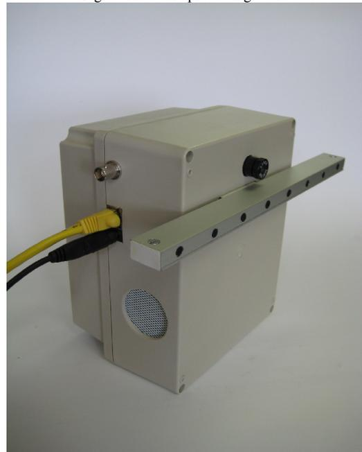
Fig. 6: The node, with apparent camera and microphone array
