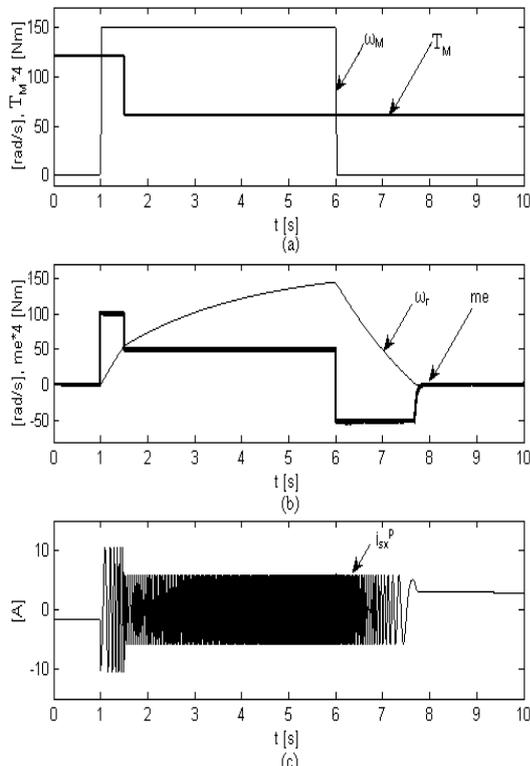
Figure 3. a) Simulation results of the predicted speed and electromagnetic torque; b) Simulation results of the speed and electromagnetic torque response of the induction motor; c) Waveform of the stator's phase current.
