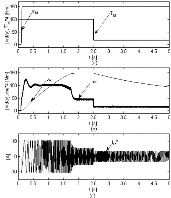
Figure 4. a) Simulation results of the predicted speed and electromagnetic torque; b) Simulation results of the speed and electromagnetic torque response of the induction motor; c) Waveform of the stator's phase current.
