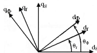
Figure 1. Phasor transformation diagram of the rotor, stator and flux measures
