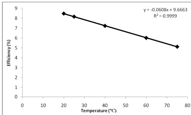
Fig. 6. Conversion efficiency variation with temperature.
