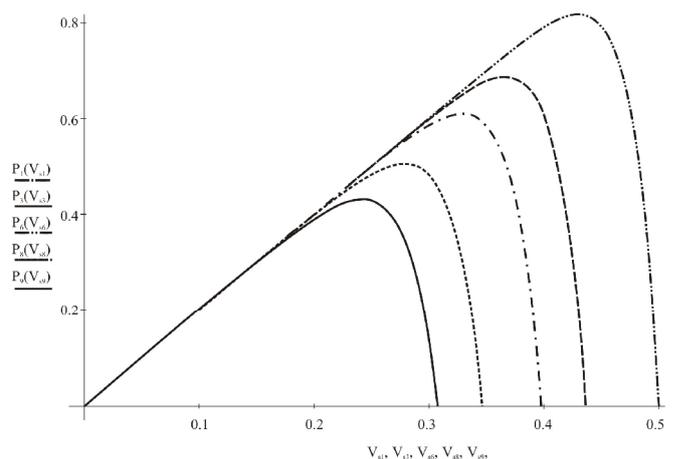
Fig.5. Set of P-V curves for a poly-crystalline silicon cell. (Values on X axis in Volts; values on Y axis in Watts)
