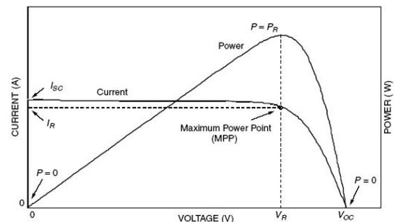
Fig. 1. I-V and P-V curves for an idealized solar cell. [5]
