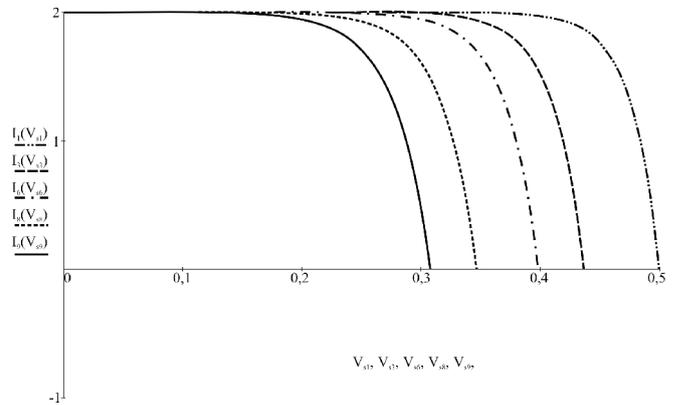
Fig. 4. Set of I-V curves for a polycrystalline silicon cell. (Values on X axis in Volts; values on Y axis in Amperes)
