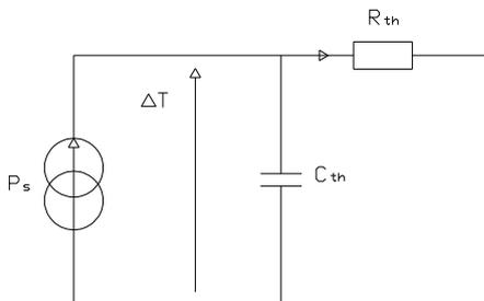
Fig. 2. Heat transfer model for a PV cell.
