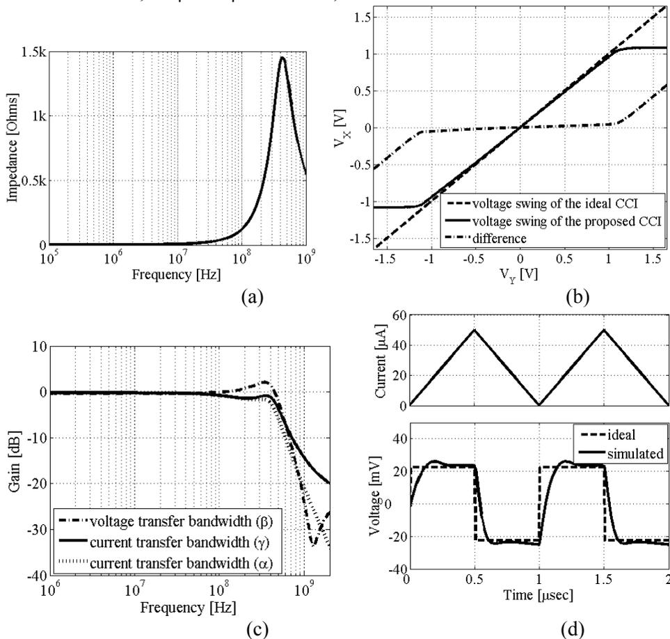
Fig. 3. (a) Variation of port X impedance value with frequency (b) Linear operation region of the proposed CMOS CCI (c) Current and voltage transfer gains (d) Time domain simulation results of the proposed lossless grounded inductance simulator
