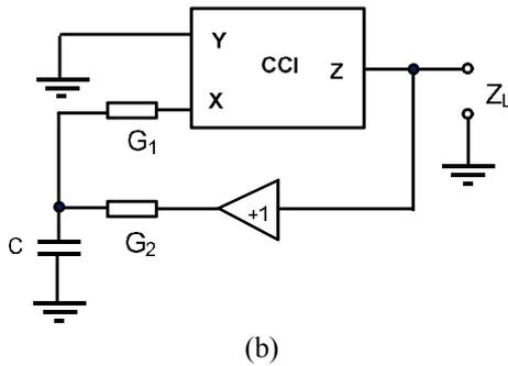
Fig. 2. The proposed inductance simulator circuits (a) lossless one (b) lossy one
