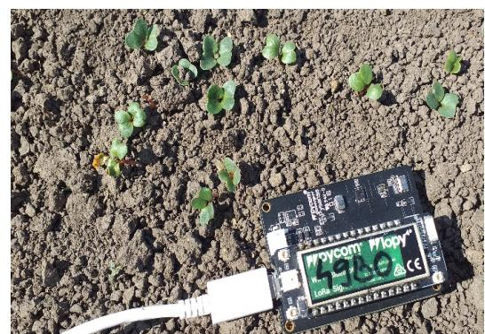
Figure 3. LoPy4 board and monitoring of radish plants
