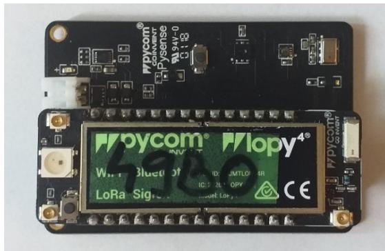
Figure 2. Pycom LoPy and Pycom Pysense boards
