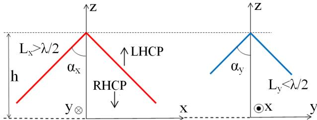
Fig. 1. Antenna geometry in xz and yz planes.
