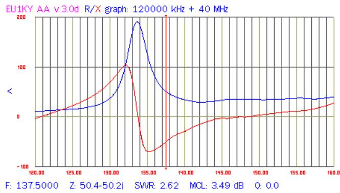
Fig. 9. The impedance components R,X measured for the capacitive (short) dipole.
