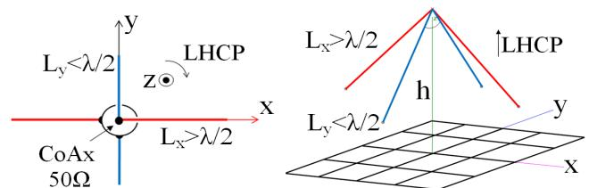
Fig. 2. Antenna geometry in xy plane and 3D.
