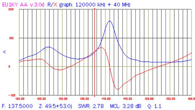
Fig. 8. The impedance components R,X measured for the inductive (long) dipole.
