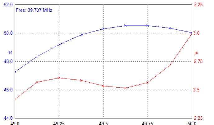
Fig. 4. The impedance  $Z=R+jX$  components for the complex conjugate impedance antenna ( $R$ -blue,  $jX$ -red).
