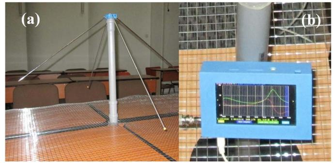
Fig. 7. The experimental setup: complex conjugate impedance 137MHz test antenna (a), EUIKY vector antenna analyzer (b).
