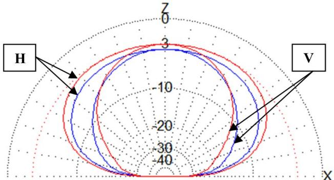
Fig. 6. Compared far field radiation patterns of the vertical (V) and horizontal (H) field components in the vertical plane: complex conjugate impedance antenna (blue), turnstile antenna (red).
