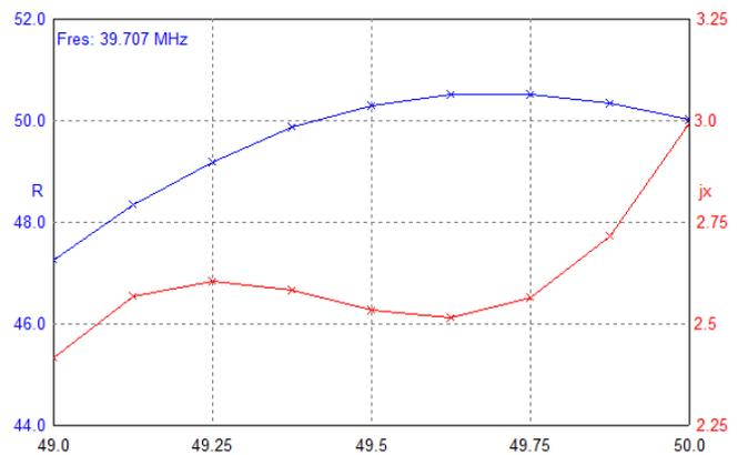
Fig. 4. The impedance  $Z=R+jX$  components for the complex conjugate impedance antenna (R-blue,  $jX$ -red).
