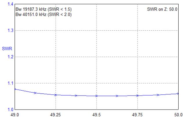
Fig. 5. The standing wave ratio SWR for the complex conjugate impedance antenna.
