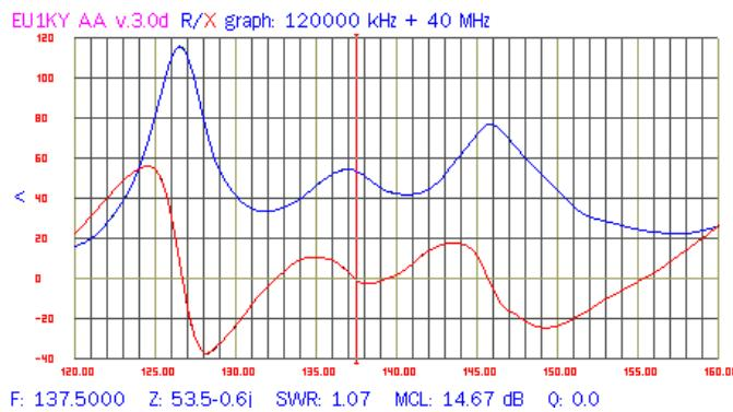
Fig. 10. The complex conjugate impedance antenna measured impedance components R,X.
