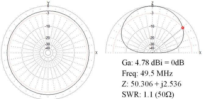
Fig. 3. Total radiation pattern of the complex conjugate impedance antenna in the horizontal and vertical planes.
