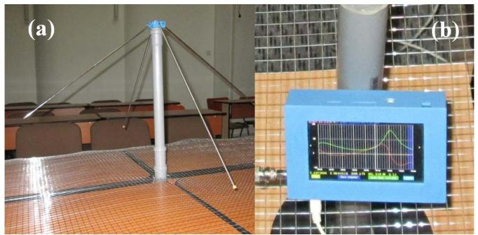
Fig. 7. The experimental setup: complex conjugate impedance 137MHz test antenna (a), EU1KY vector antenna analyzer (b).
