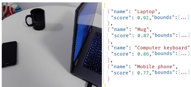
Fig. 3. Example of results delivered by the feature extraction component (JSON format). Each object is described with its name, confidence score, and an array of points for localization in the image.
