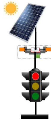
Fig. 1. Design of the traffic light with sun tracking system
