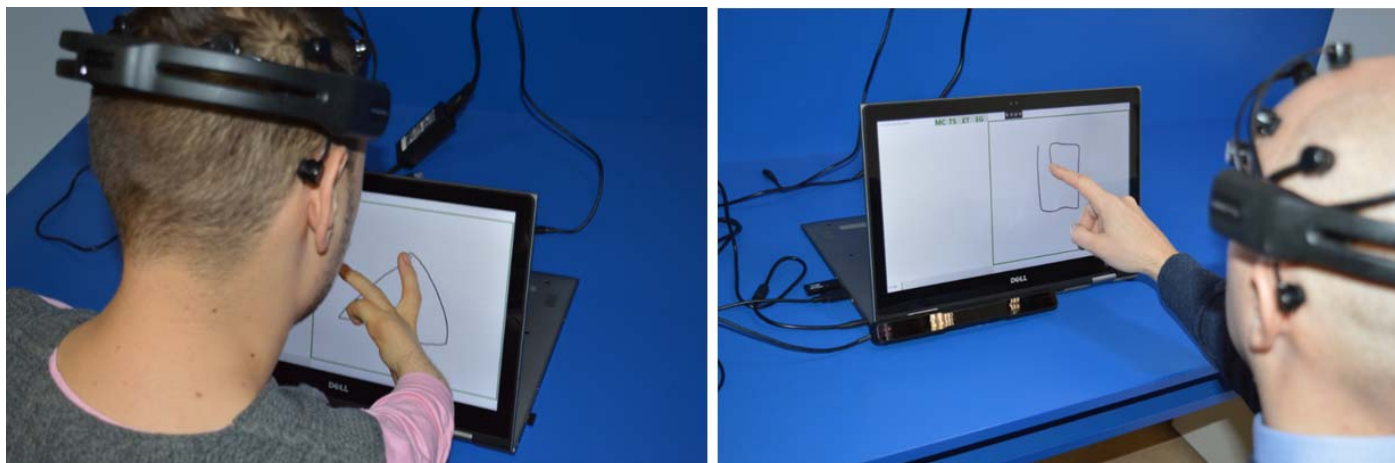
Fig. 5 - The VERGE system employed in a practical experiment for collecting multimodal data (voice, touch gesture, eye gaze, and EEG) from participants with motor impairments (left) and without impairments (right).
