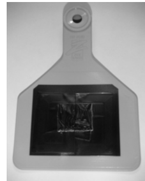
Figure 6. The label transponder attached to the animal's tag.
