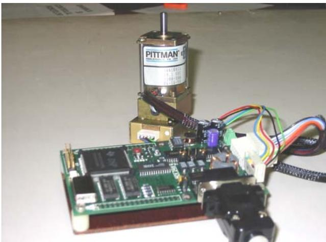
Figure 3. MCK240 system with BLDC motor
