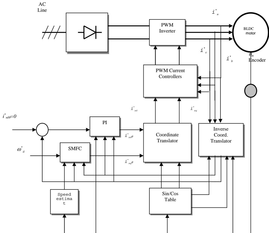
Figure 2. SMFC controller for BLDC motor drive
