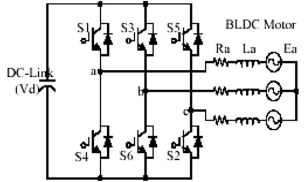
Figure 1. Current controlled PWM inverter
