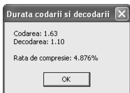
Figure 5. The window containing the parameters of the encoding-decoding process.
