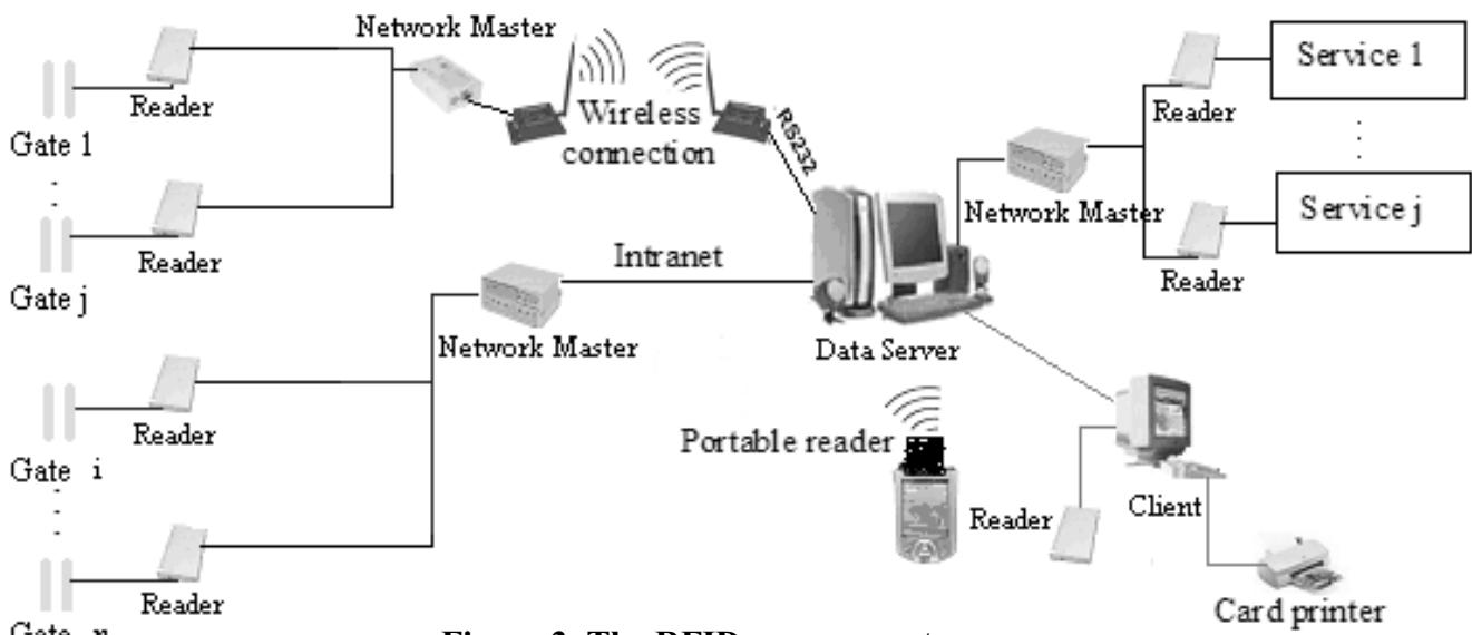
**Figure 3. The RFID campus system**
