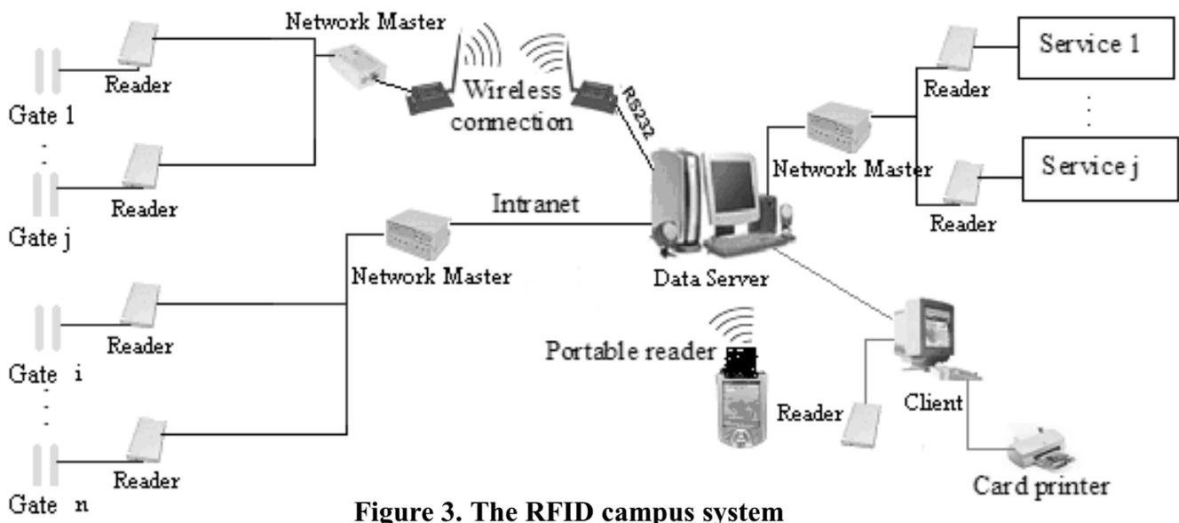
**Figure 3. The RFID campus system**
