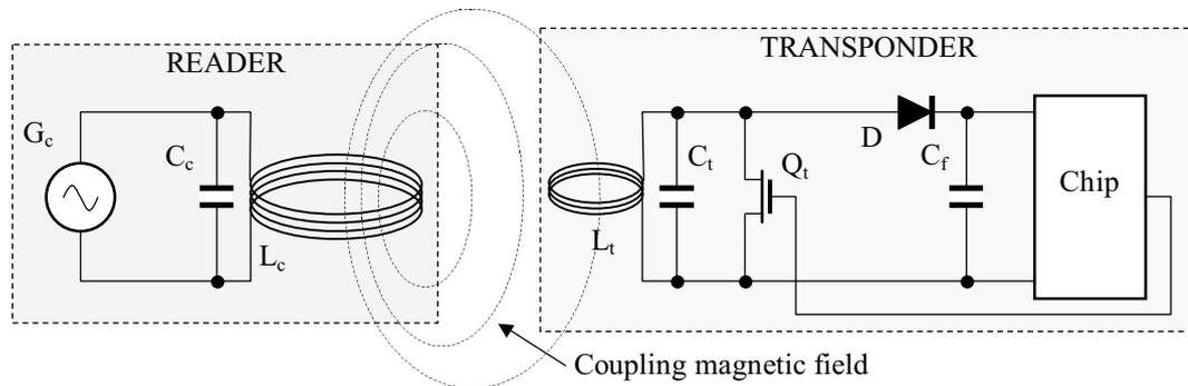
**Figure 1. Energy and data transfer between reader and transponder**
