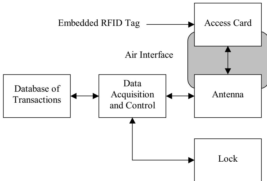
**Figure 2. The access control system for one gate.**
