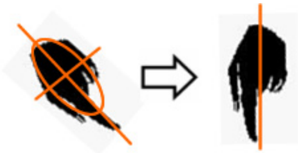
Figure 7. Blob rotation based on the axis of the ellipse of inertia.
