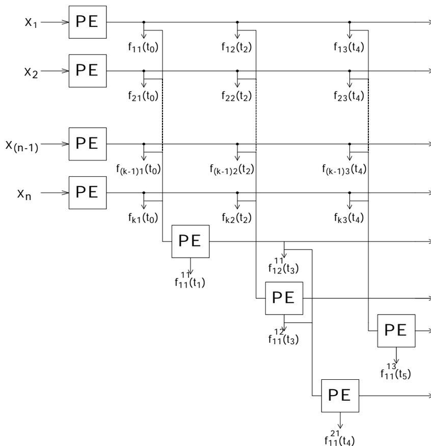
Figure 3. Structural diagram of interaction of information flows in parallel-hierarchical computational structure.
